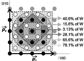
The crystal basis of our super-cell contains 32 atom in both A (solid circles) and B (open circles) (001) planes. The gray solid circles belong to other (adjacent) super-cells. The dashed contours define considered interfaces between tungsten (W) wire and niobium (Nb) matrix in investigated lamina models of different atomic concentration of W.
